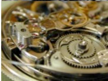
Ultra-flat column wheel of the split second mechanism
