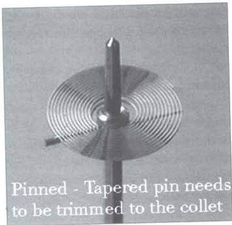
Spring and collet are being pinned together with a brass tapered pin.
