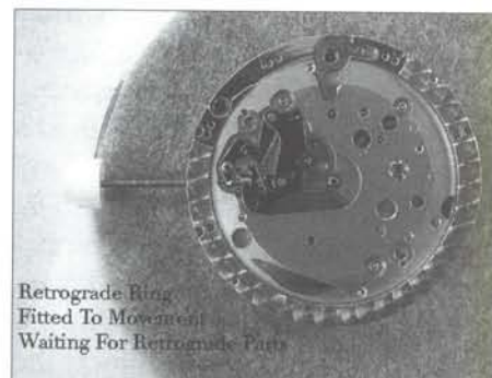
Plated, Cleaned & Ready For Assembly
