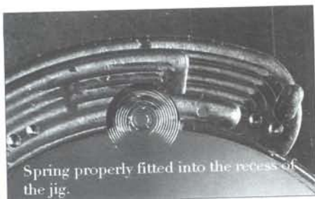
Colleted spring placed into jig to determine correct size for use in movement. It is too large currently.
