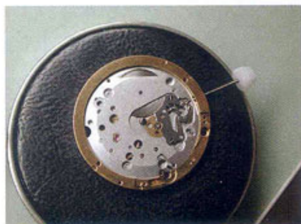
Above: Spacer ring is placed on the movement and held in place by the stem.
