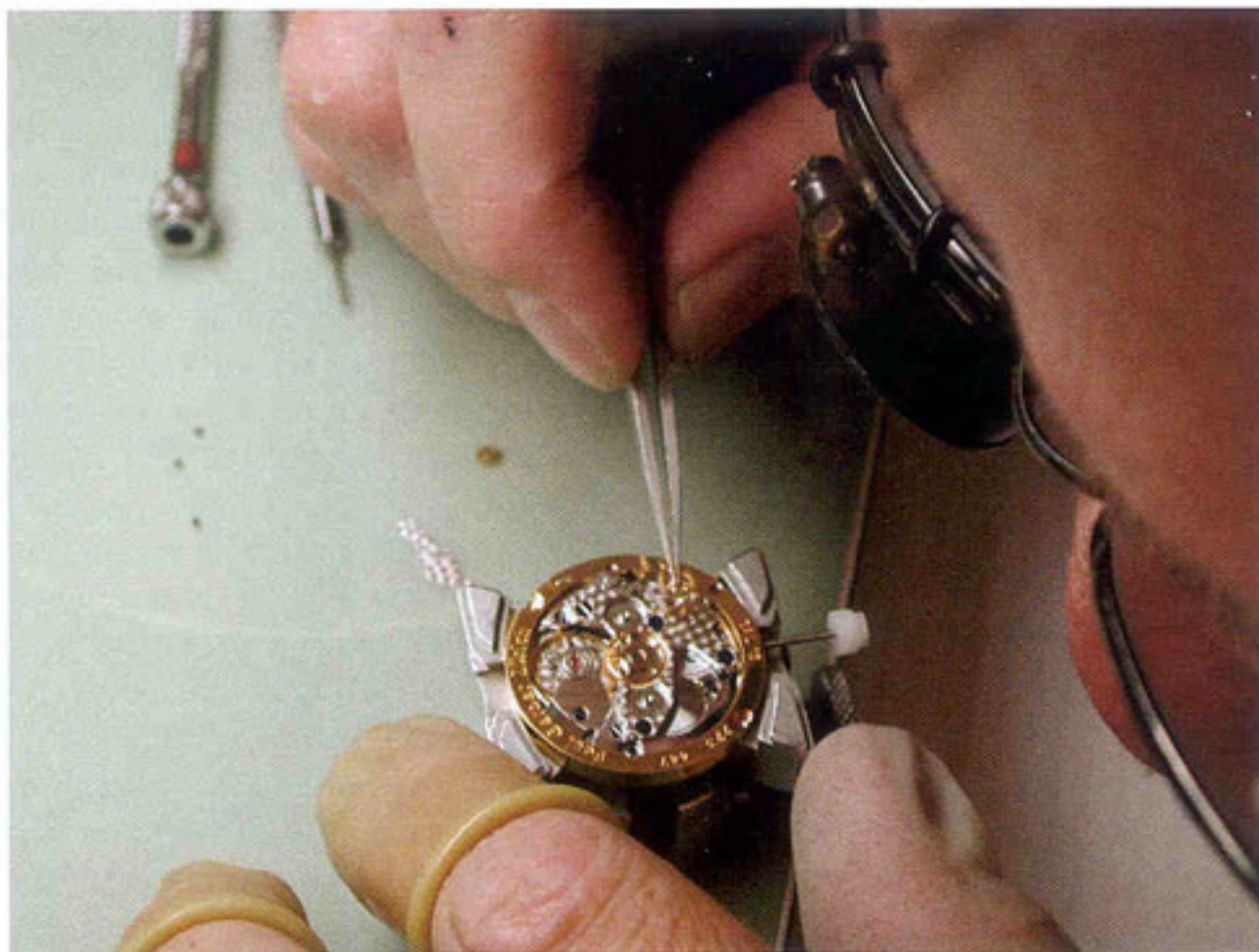
Assembling automatic train. Retrograde spring is colleted and pinned.
