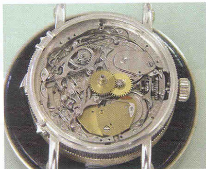
The workings of the minute repeater
