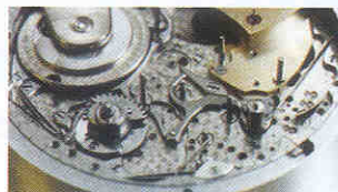
Modifications made to the main plate to fit the tourbillon
