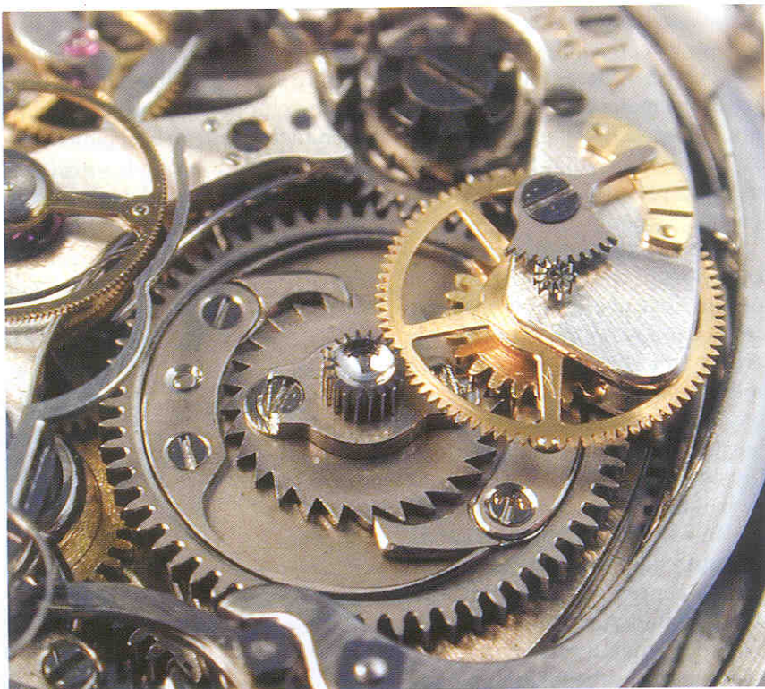
Above: Close-up of mainspring section of movement and one of the power reserve indicators.
