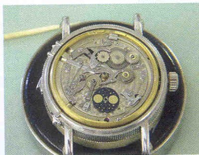
The perpetual calendar mechanism
