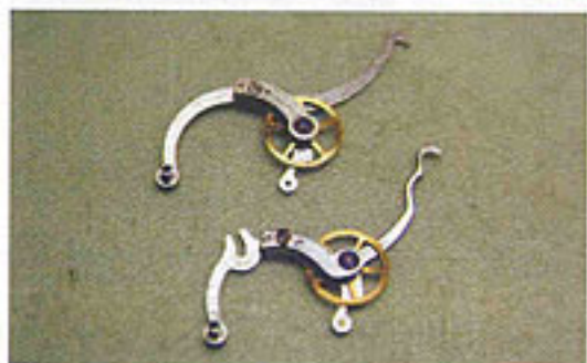
Column wheels (top) and levers (above) were tested and discarded if they didn't meet Gerber's precise specs.
