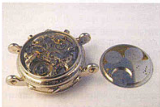
Top: Chronograph with dummy bridges and plates; above, completed watch next to a dummy plate
